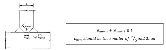
Figure 1. Effective full penetration of T-butt welds after EN 1993-1-8.
