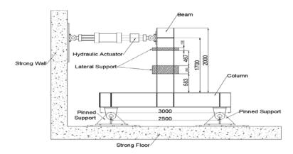
Figure 2. Test set-up based on the SAC protocol. All numbers in millimeter [mm].
