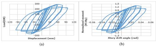
Figure 8. Hysteresis behaviour of connection in specimen 1: (a) load-displacement curve, (b) Normalised moment versus story drift angle.
