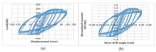
Figure 9. Hysteresis behaviour of connection in specimen 2: (a) load-displacement curve, (b) Normalised moment versus story drift angle.
