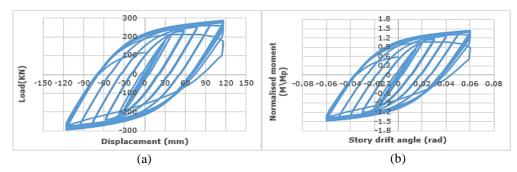
Figure 10. Hysteresis behaviour of connection in specimen 3: (a) load-displacement curve, (b) Normalised moment versus story drift angle.
